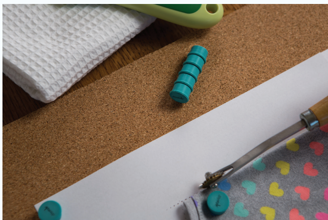
Pattern maker cork side of mat, pin needle tracer and stackable magnets.
